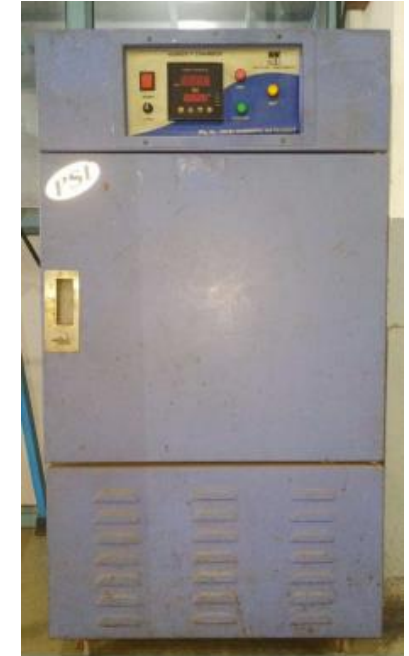
Humidity Chamber Inner S.S. Outer M.S.
